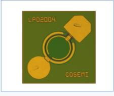
Cosemi's LPD2004 is a mesa-structured, InGaAs/InP-based PIN photodiode offering high responsivity, low dark current and low capacitance for high bandwidth, high performance optical receiver designs.
